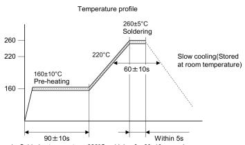
Peak temperature: 260±5°C for within 5 seconds. Soldering temperature: 220°C or higher for 60±10 seconds. Pre-heating temperature: 160±10°C for 90±10 seconds. Quartz crystal units which is put on PCB shall be through reflow soldering furnace twice with the condition shown above.
