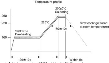
Peak temperature: 260±5°C for within 5 seconds. Soldering temperature: 220°C or higher for 60±10 seconds.
